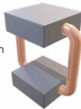
Fluid flow circulates in a tubular serpentine between evaporator and condenser areas. The riser and downcomer of the circuit can either be adiabatic or participate to heat transfer. They may also include bends and turns.
